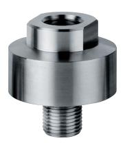
Diaphragm seals are designed to isolate the sensing element of pressure gauges and pressure switches from process fluids that may be corrosive, viscous, sediment-laden and/or with a high temperature. The diaphragm is welded to the body to ensure that the filling fluid and the process medium are completely separated. Threaded connections allow their use in all applications where the compact size of the assembly is important and where instruments with a 2,5" (63 mm) diameter are required.
